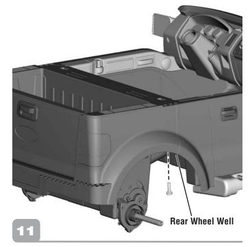
• Insert a screw up through both rear wheel wells and into the cargo bed. Tighten the screws.
